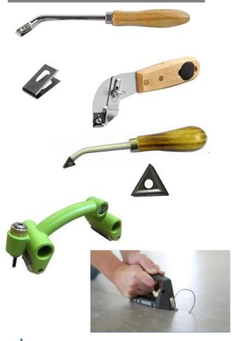
Triangular tools that are branded as corner scrapers are an aggressive gouging tool rather than a cutting tool. If used for grooving they can be difficult to control particularly on a homogenous chip vinyl.
