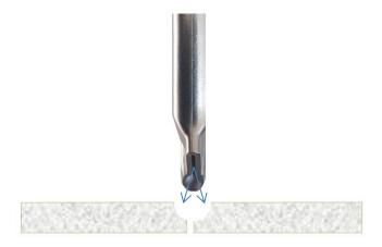
Hot air stream directed into the groove
